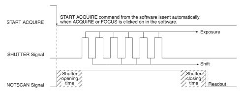
Figure 22. Free Run Timing Diagram
